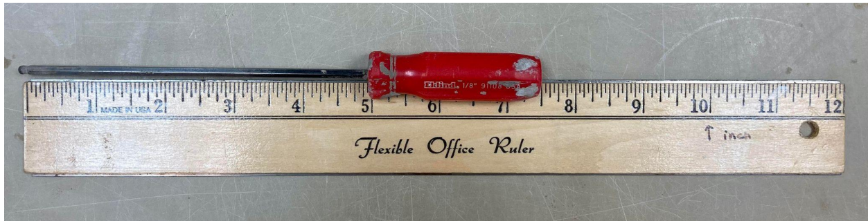
Figure 2: Use a 1/8" in ball end hex screw with a 5 in head to insert a 10 cm Rhizon filter piece.
